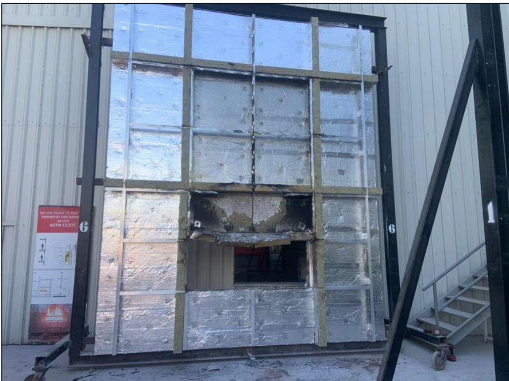
Picture 22: Specimen during dismantling after removal of the external cladding panels.
