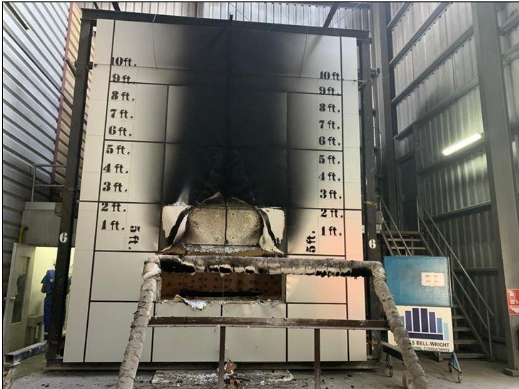
Picture 21: The specimen at the end of the observation period and end of the NFPA 285 test.
