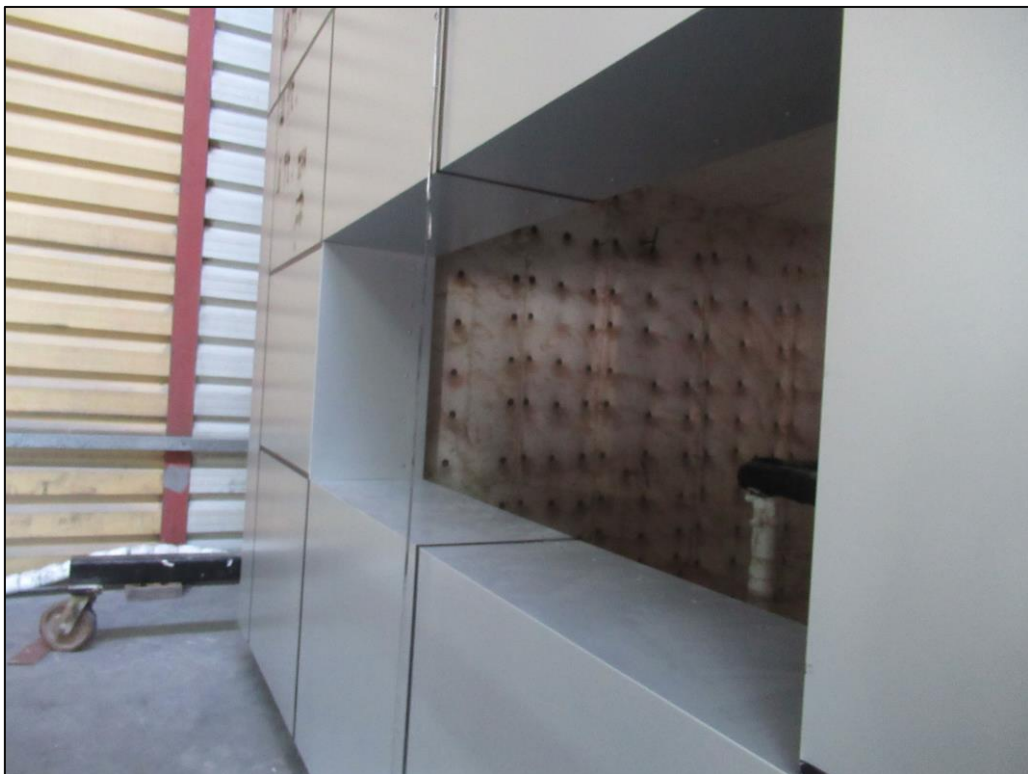
Picture 10: A view of the window opening termination of the test specimen.
