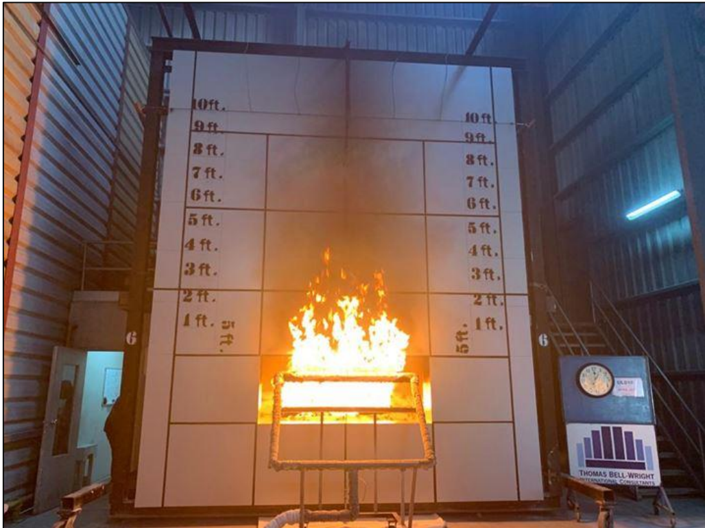
Picture 13: The specimen at 5:00 minutes and when the window burner was ignited.
