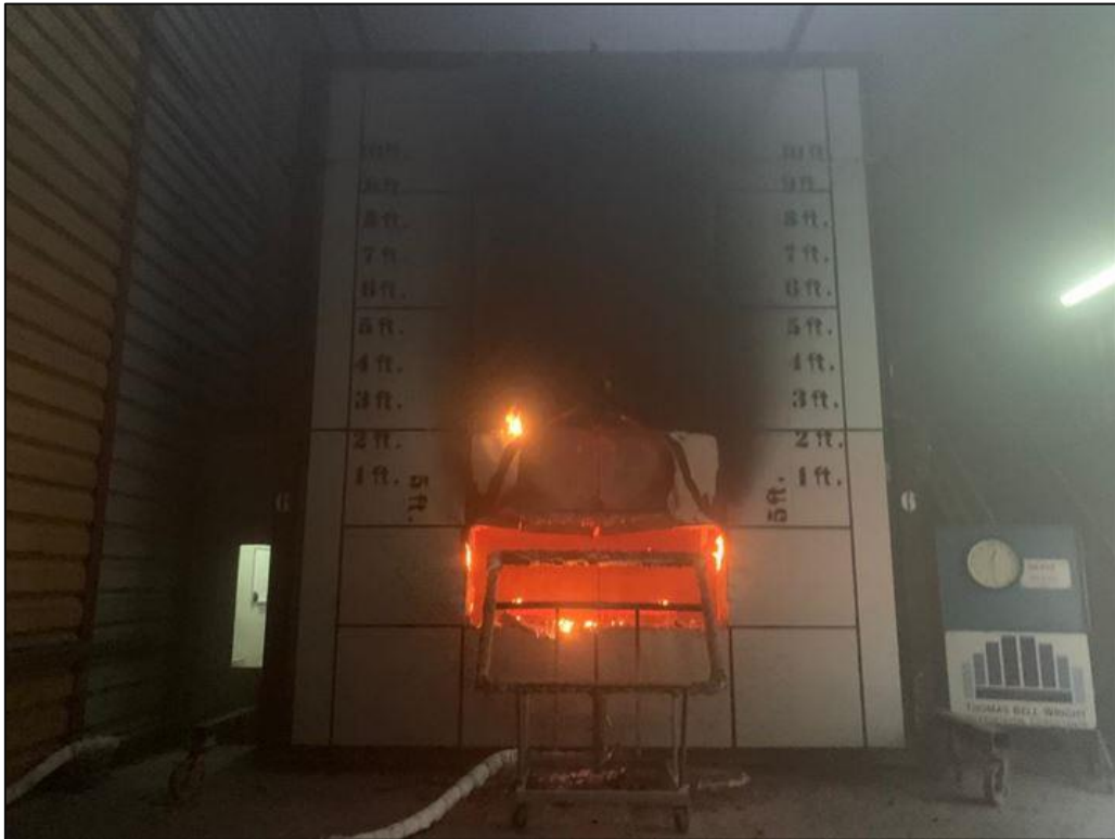
Picture 19: The specimen immediately after the gas was shut off, starting the observation period.
