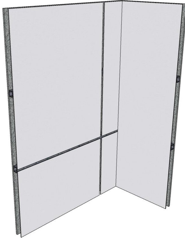
Drawing 1: Isometric view of the Specimen. The ACP assembly was tested with an 80mm air gap.
