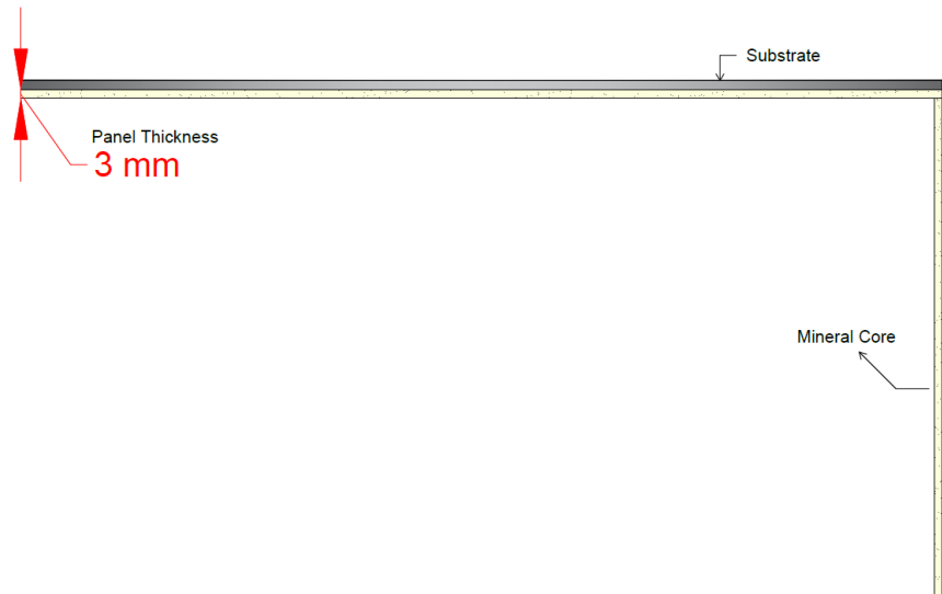
Drawing 3: Top view of the mounted specimen without airgap. All dimensions are in millimeters (mm)
